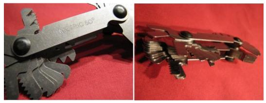
**Fig. 2.4a:** Metric / English combination thread gauge. (I doubt that you will ever need this. If you find a cheap one, perhaps, go for it. I got this one for a few dollars at Max shop.)
